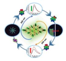
A 3D metal-organic framework (MOF) consisting of an anthracene moiety is reported, which is the first example of a MOF exhibiting both direct chemiluminescence and dual tunable photoluminescence. The material is explored as a selective visual sensor for probing hydrogen peroxide, a dual sensor for aromatics, and a quantitative sensor for nitroaromatics.
