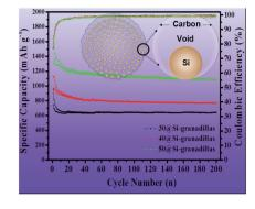
A green and facile way to synthesize an integrated outer carbon-layer-coated granadilla-like silicon/carbon composite is presented. The material is composed of inside carbon network supported yolkshell silicon nanobeads. The simple fabrication makes it promising to serve as improved anode material for lithium-ion batteries.
