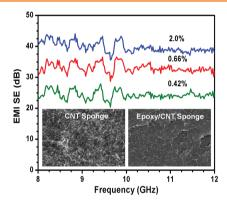
High-performance electromagnetic interference shielding epoxy nanocomposites are prepared using a preformed highly porous and electrically conductive CNT sponge. The CNT sponge acts as the three-dimensional conducting framework and as effective reinforcement. Only 0.66 wt% of CNT sponge leads to an outstanding EMI shielding effectiveness of around 33 dB in the X-band, and vast increments in the flexural strength and tensile toughness are achieved.
