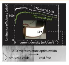
An indium-free anode is developed by a ZnO-SnO<sub>2</sub> combinatorial study. The optimized Zn-Sn-O (ZTO) compound presents a void-free amorphous microstructure, low roughness, high electron mobility, and <5% visible range absorptance. Large-area (41 cm²) flexible organic light-emitting diodes (OLEDs) fabricated with a ZTO/grid anode outperform those with a Sn-doped In<sub>2</sub>O<sub>3</sub> (ITO)/ grid anode, confirming the industrial application potential of ZTO.
